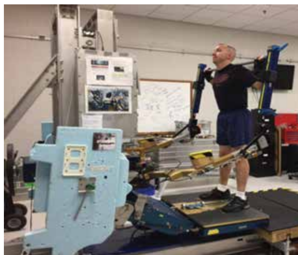
FIGURE 2: Astronaut Randy Bresnick training on an Advanced Resistive Exercise Device (ARED), which helps maintain muscle strength
