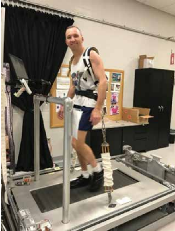
FIGURE 3: Astronaut Randy Bresnick on a Treadmill with Vibration Isolation and Stabilization System (TVIS), which helps maintain muscle and bone strength
